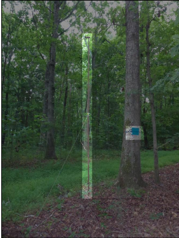
Figure 3-4. Sampling flyways. Bat detector deployed along a forest path that serves as a flyway for bats. Detector is attached to a tree, whereas the microphone is elevated on a pole and positioned to the side of the path and away from the immediate acoustic shielding of the tree; both are highlighted in the lighter shaded areas of the image. Always consider whether vehicles or people may collide with detectors and other equipment when sampling along flyways like roads or hiking paths. © Alexander Silvis.
